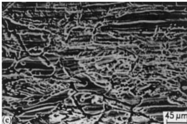
Fig. 4 (a) to (c) SEM of laser-melted AISI 316 SS (898 K-50 h-25% CW): (a) laser-melted zone, desensitized zone, and unaffected base metal; (b) desensitized zone showing step structure with globular carbides distributed discontinuously; and (c) desensitized zone/base metal interface showing disappearance of ditch structure and formation of globular carbides
